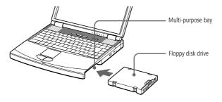
When the computer is in System Suspend or System Hibernation mode, you cannot insert a disc.
